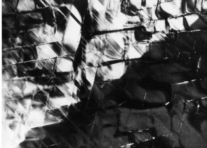
Figure 7.3: Lorentz electron micrograph of a  $\text{Sm}(\text{Co,Fe,Cu,Zr})_z$  magnet. The magnetic domain wall between two domains with opposite magnetization (bright and dark cells) is pinned on the precipitation structure [87].
