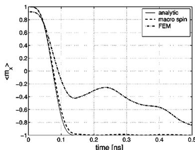
FIG. 4. Analytical and numerical solutions of Landau–Lifshitz–Gilbert equation. Plot of  $\langle m_x \rangle$  vs time:  $h_a = 1.5 \times h_{SW}$ ,  $D_x = 1.2 \times 10^{-3}$ ,  $D_y = 0.0175$ , and  $D_z = 0.9763$ .
