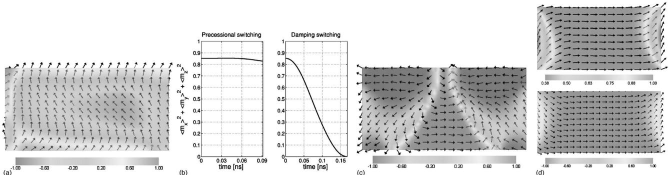
FIG. 3. Numerical results: (a) precessional switching: magnetization vector field at  $t = t_0$ ; (b) plot of  $\langle m_x \rangle^2 + \langle m_y \rangle^2 + \langle m_z \rangle^2$  vs time in the interval  $(0, t_0)$  for damping (right) and precessional switching (left); (c) damping switching: magnetization vector field at  $t = t_0$  (the applied field strength is  $H_a = 19.51$  kA/m), and (d) S state (top), C state (bottom).
