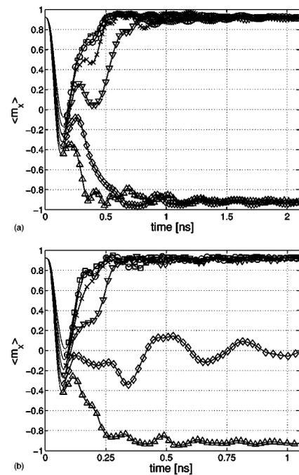
FIG. 5. Numerically computed  $\langle m_x \rangle$  as a function of time: (a)  $S$  state, (b)  $C$ -state initial condition. Symbols: ( $\square$ ) stands for  $h_a = h_{SW}$ ; ( $\circ$ ) for  $h_a = 1.1 \times h_{SW}$ ; ( $\times$ ) for  $h_a = 1.2 \times h_{SW}$ ; ( $\nabla$ ) for  $h_a = 1.3 \times h_{SW}$ ; ( $\diamond$ ) for  $h_a = 1.4 \times h_{SW}$ ; and ( $\triangle$ ) for  $h_a = 1.5 \times h_{SW}$ .
