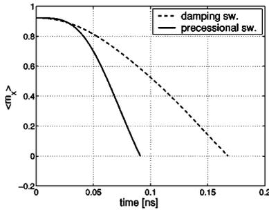
FIG. 2. Numerical results: comparison between damping (dashed line) and precessional (solid line) switching: time for average  $m_x$  component to reach zero from the starting configuration for  $H_a = 19.51$  kA/m.
