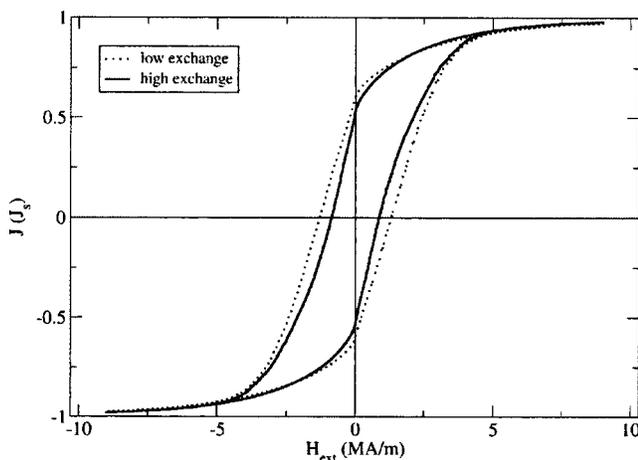
FIG. 2. Hysteresis loops for FePt particles calculated using the modified Stoner–Wohlfarth model for high exchange ( $A = 1.4 \times 10^{-11}$  J/m) and low exchange ( $A = 0.4 \times 10^{-11}$  J/m).
