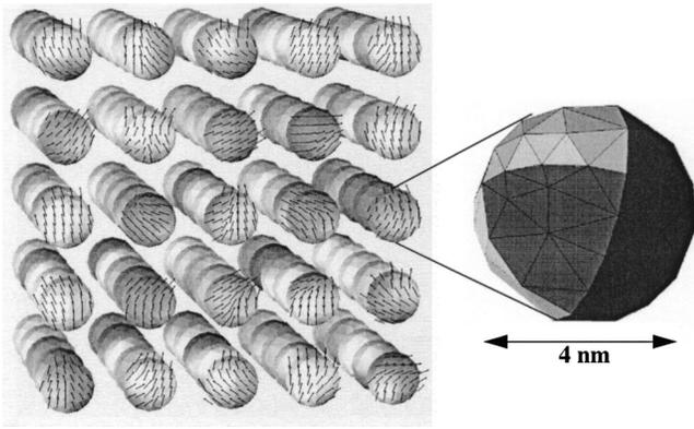
FIG. 1. Finite element model of self-assembled FePt particles. The arrows show the magnetization distribution for zero applied field. Owing to the exchange interactions between the grains which form an FePt sphere, the magnetization arranges nonuniformly. The enlarged sphere on the right-hand side shows the surface of the finite element mesh. The different colors correspond to crystallites with different easy axis direction.
