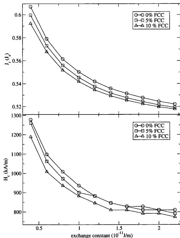
FIG. 4. Hysteresis properties as a function of the strength of the exchange interactions within a particle agglomerate. Top: Reduce remanence as a function of the exchange constant. Bottom: Coercive field as a function of the exchange constant. The error induced by the finite field step is in the size of the symbol.
