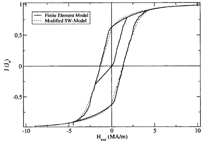
FIG. 3. Comparison of the hysteresis loops calculated from the modified Stoner–Wohlfarth model ( $A = 0.4 \times 10^{-11}$  J/m) and the finite element model ( $A = 0.1 \times 10^{-11}$  J/m). In addition a recoil curve calculated with the finite element model is shown.
