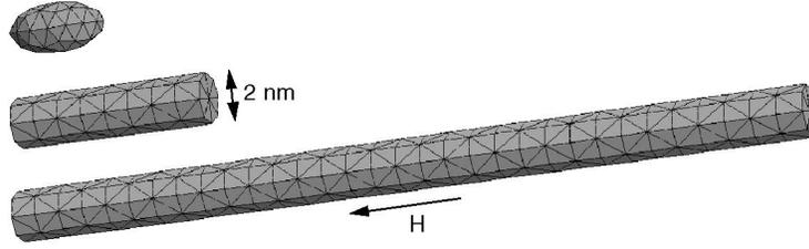
Figure 1: Finite element models of the particles used for the simulation of thermally activated switching.
