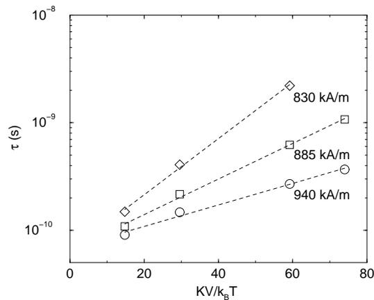
Figure 2: Relaxation time as a function of  $KV/(k_B T)$  for different applied fields.
