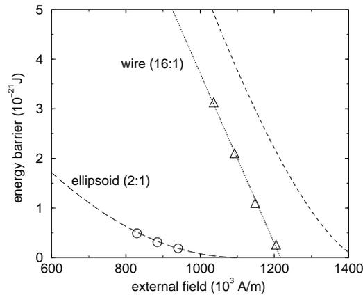
Figure 3: Activation energy as a function of the applied field. The open symbols give the numerical values. The dashed lines give the analytical results according to equation (20) and (23). The dotted line is linear fit of the numerical values for the nanowire.
